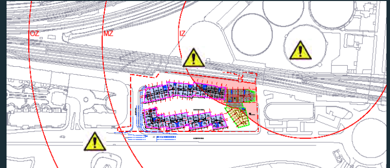
Site Plan with significant hazards indicated
